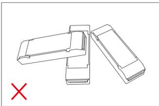
Please do not stack the products. The distance between two products should be  $\geq 15\text{cm}$  so as not to affect heat dissipation or the lifetime of the products.
