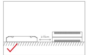
Note: The temperature within the installation area should be within the working temperature range of the products. Please do not install products inside LED fixtures to avoid temperature exceeding the working temperature that may affect the product lifetime.
