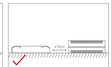
Please do not stack the products. The distance between two products should be  $\geq 15\text{cm}$  so as not to affect heat dissipation and the lifespan of the products.
