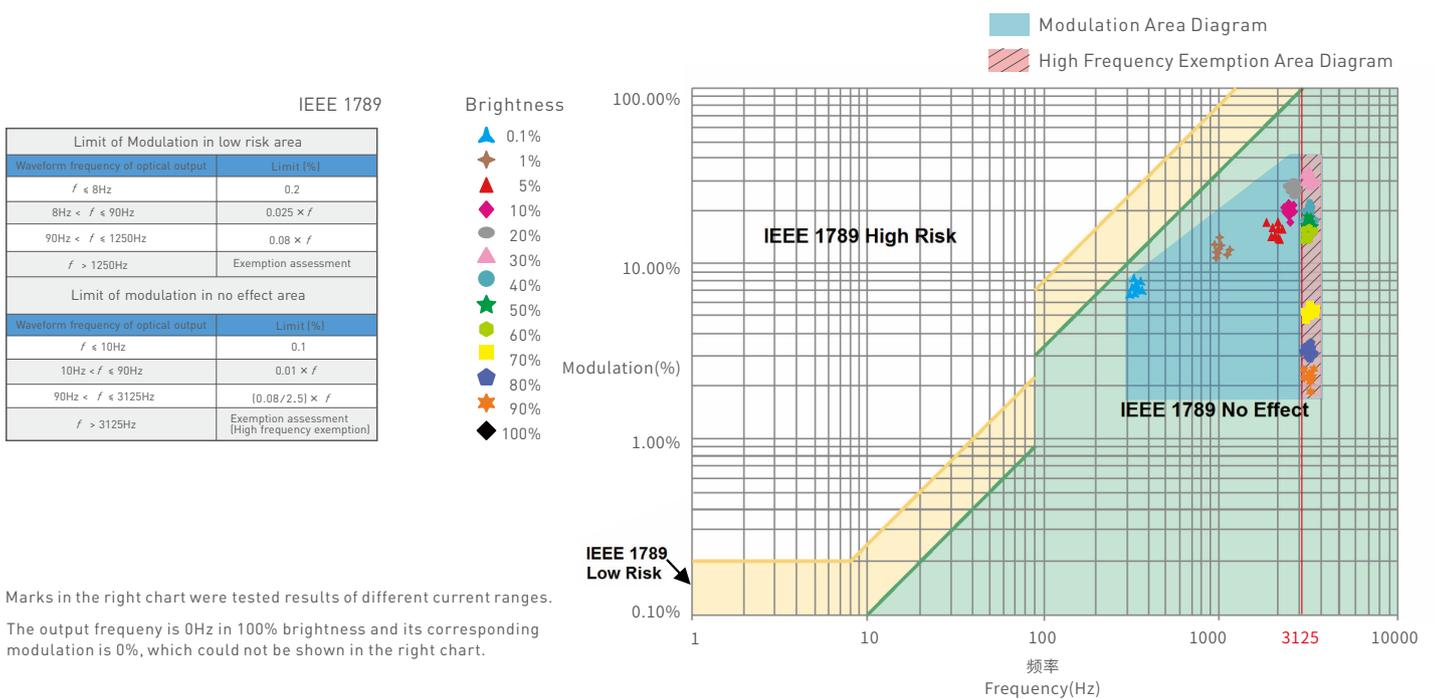
Marks in the right chart were tested results of different current ranges. The output frequency is 0Hz in 100% brightness and its corresponding modulation is 0%, which could not be shown in the right chart.
