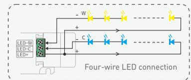
\* Adopting constant power program design, it keeps the same brightness in color temperature dimming, and twice the rated power load can be connected.
