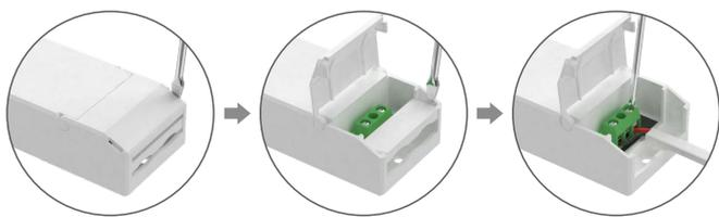
1. Put the head of a screwdriver on the side of the housing to pry up both the protective cover and wire fixing board. Then remove the wire fixing board and connect to the wires as wiring diagram shows.
