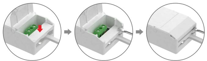
2. Install the wire fixing board and press it down. Then snap on the protective cover while pressing the wire fixing board with a small flat-head screwdriver
