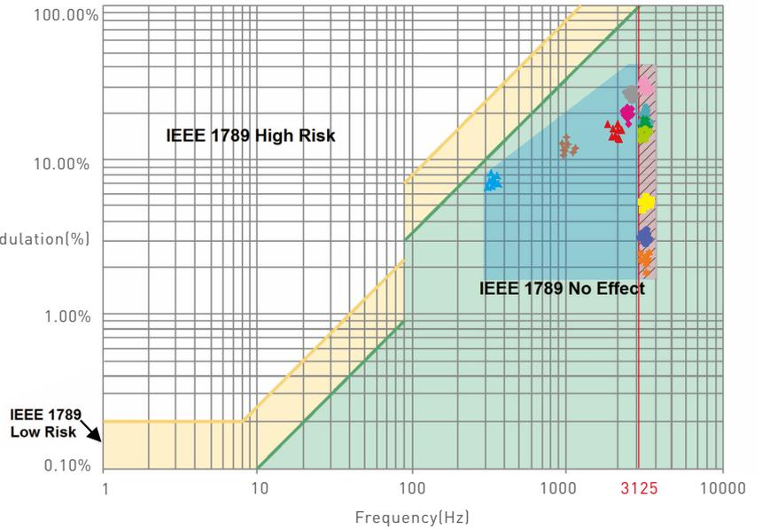
Marks in the right chart were tested results of different current ranges. The output frequency is 0Hz in 100% brightness and its corresponding modulation is 0%, which could not be shown in the right chart.
