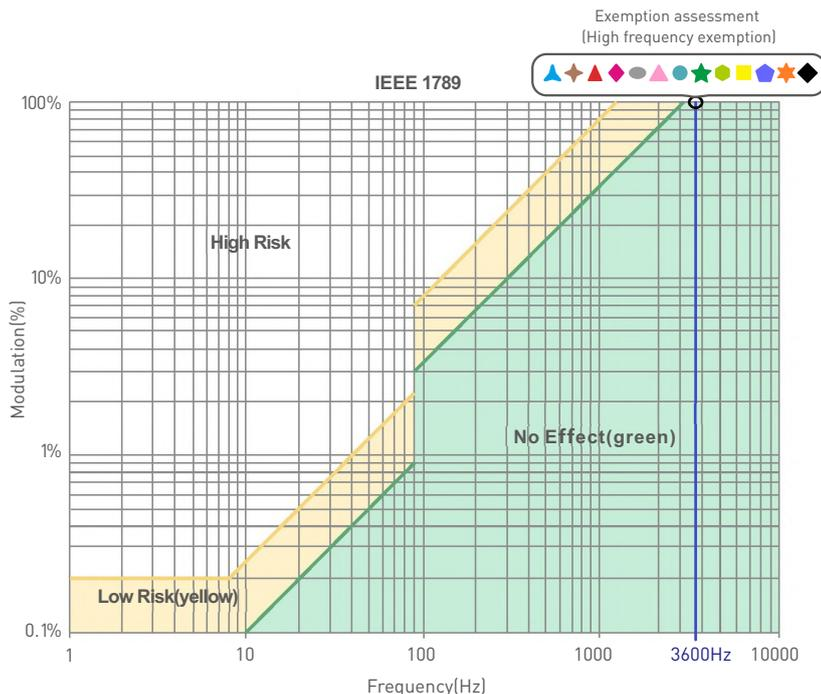
Marks in the right chart are tested results of different current levels. The output frequency is 0Hz in 100% brightness and its corresponding modulation is 0%, which could not be shown in the right chart.
