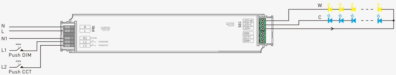
4. Brightness and color temperature adjustment simultaneous.
