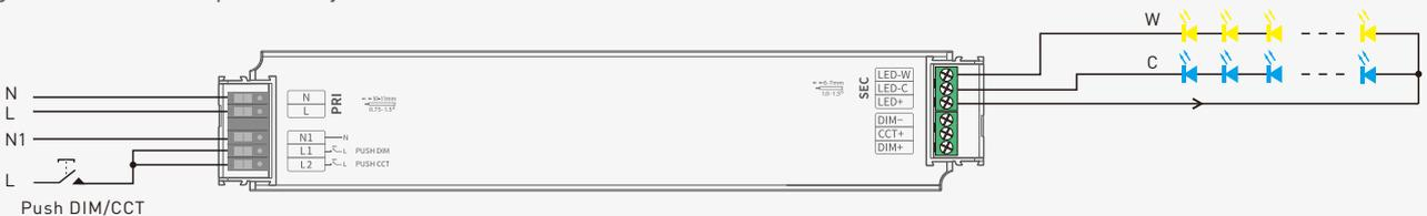
\* Dimming interface priority: First 0-10V, next Push DIM/CCT.
