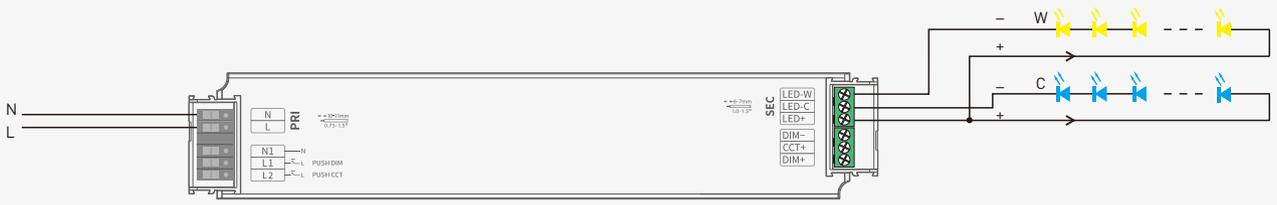
\* Adopting constant power program design, it keeps the same brightness in color temperature dimming, twice the rated power load can be connected.
