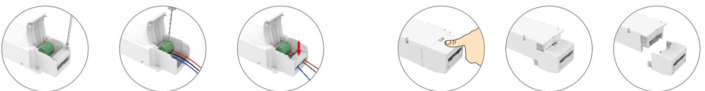
Use a screwdriver to pry up the protective housing at the edge of the wire fixing board. Then connect to the wires as the diagram shows and press down the wire fixing board.
