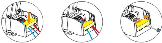
Push the wire pressing board to fix the wires.
