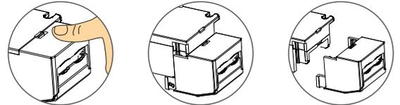
Break off the bottom left and right to remove the protective cover.
