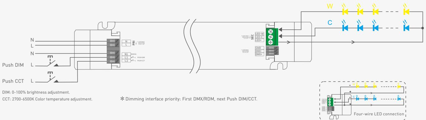
\* Adopting constant power program design, it keeps the same brightness in color temperature dimming, twice the rated power load can be connected.
