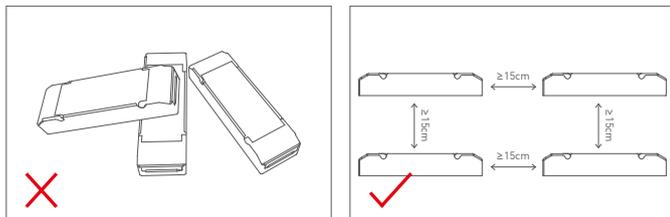
Please do not stack the products. The distance between two products should be  $\geq 15\text{cm}$  so as not to affect heat dissipation and the lifespan of the products.
