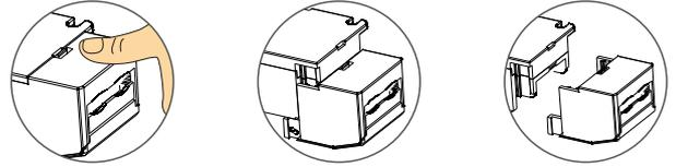
Break off the bottom left and right to remove the protective cover.
