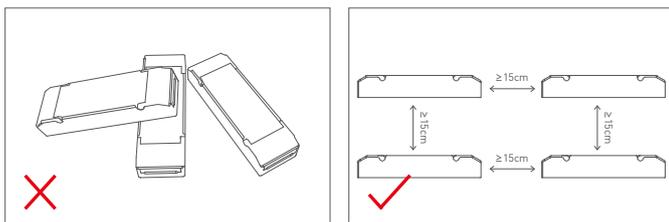
Please do not stack the products. The distance between two products should be  $\geq 15\text{cm}$  so as not to affect heat dissipation and the lifespan of the products.
