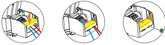
Push the wire pressing board to fix the wire.
