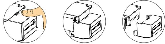
Break off the bottom left and right to remove the protective cover.
