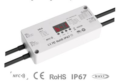
The HD4 is a high-performance LED constant-voltage controller with IP67 waterproof rating. It receives standard DALI protocol signals and is compatible with all DALI systems on the market, specifically designed for precise control of LED lighting fixtures. Featuring 4 channels, it delivers a maximum output current of 6.4A and a maximum output power of 1536W, enabling stable operation of various LED constant-voltage fixtures.
