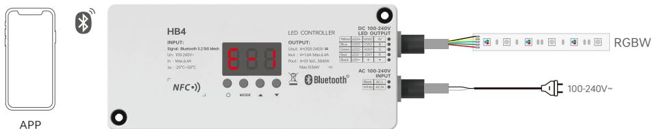
5. Adaptive Synchronization: Automatically selects operating modes to ensure consistent lighting effects across multiple devices. When devices are not networked, AC synchronization is enabled (multiple controllers on the same circuit powering up simultaneously can synchronize via AC dynamic mode). When devices are networked, Bluetooth synchronization is enabled (group playback of lighting effects synchronizes devices within the group via Bluetooth dynamic mode).
