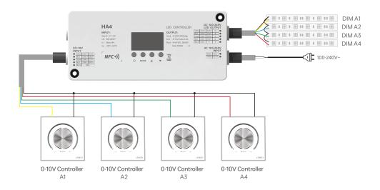
2.Connect four dimmable lights simultaneously, with one dimmer controlling all four lights at once. Set the dimming mode to "Dimming" in the NFC Lighting app.
