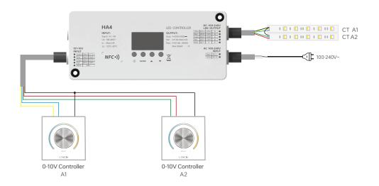
4.Connect two color temperature lights simultaneously, with one controller managing both lights at the same time.
